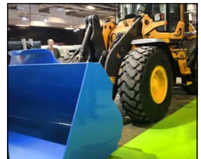
New designs: working with carbon fiber to make the front loader bucket lighter to carry a heavier load and operate for less.
